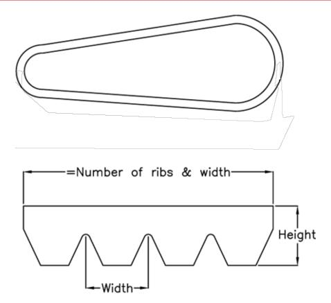
$\begin{array}{ll} \text{Datum Llength} = 1992 \\ \text{Height} &= 3.5 \\ \text{Number of ribs} = 16 \\ \text{Pitch} &= 2.34 \\ \end{array}$
